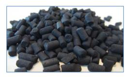
EC-102 chemical media is designed to provide the superior performance against acid contaminants. EC-102 media removes contaminant gases by chemisorption using adsorption and chemical reaction (acid-base). Gases are trapped within the pellet and converted into harmless solids that remain in the pellet, eliminating the possibility of desorption and release back into the airstream.
