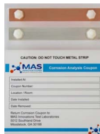
Figure 3 – Corrosion Coupon with Copper and Silver
